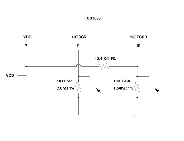
Leave place holder but do not install bypass capacitors.
